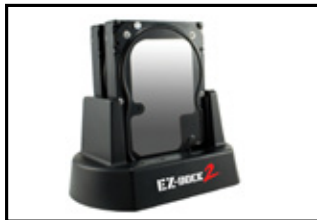
Inserted with Two 3.5" SATA H.D.D.
