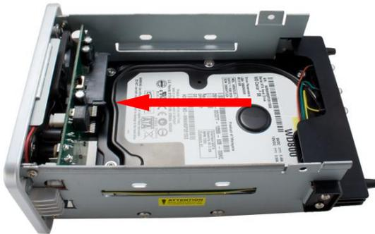
3. Place the second HDD into the top tray. Push the HDD to connect the SATA connector.
