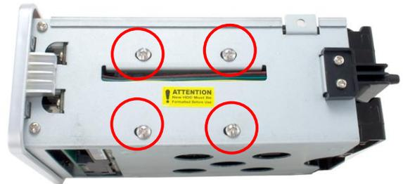
5. Push the tray into the aluminum case. Screw in the rear panel and enclosure together.
