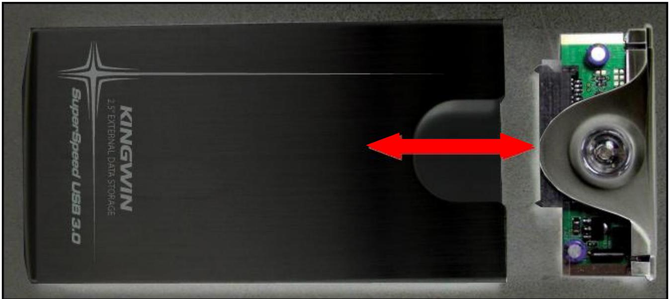
3. Connect the 2.5" H.D.D. to the SATA connector. Make sure the drive is tightly connected.
