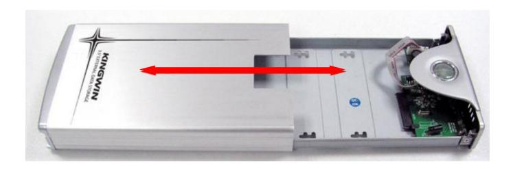
3. Connect the HDD to the SATA connector. Make sure the drive is connected tightly.
