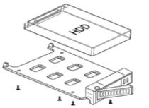
3. Ensure the SSD/HDD screw onto the tray and gently insert back to KF-261-BK
