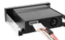
2. OR Insert Molex 4P Power + SATA 7P cable to the KF-252-BK, then another end connect to PC power plug, and motherboard or the SATA RAID card
