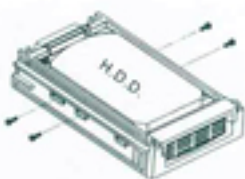
Fig.4 Screw the H.D.D. on
