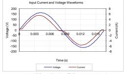
Input AC Current Waveform (ITHD = 13.76%, 50% Load)
